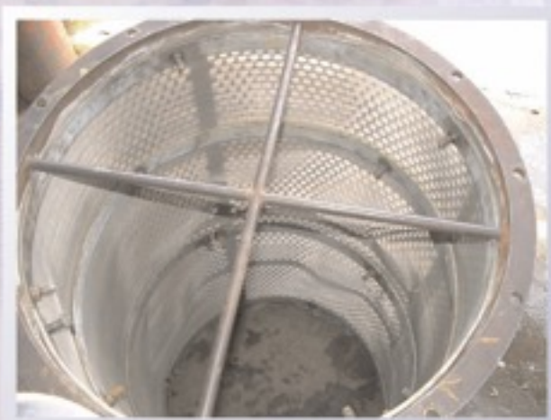
Fine (60) mesh screen is perfectly clean after high velocity flushing superheater for 4 hour acceptance run.
